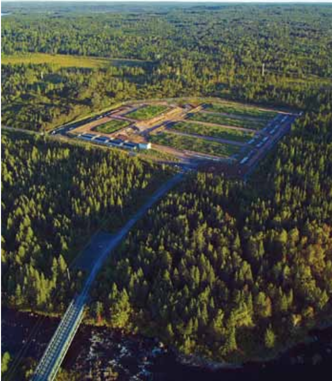
Abydoz Engineered Wetland Facility constructed in 2006 serving the Towns of Appleton and Glenwood, with a design population of 1,800.
